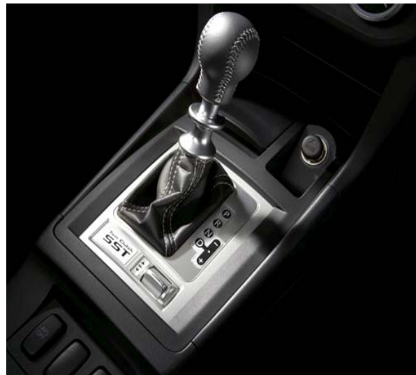
The TC-SST console mounted shifter was engineered to mimic the feel of a crisp-shifting manual transmission shifter. The mode selector is seen to the lower right. (Right-hand drive model shown.)
