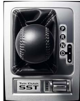
The TC-SST can be shifted manually with either the console mounted shifter or the magnesium steering wheel shifter paddles (below).
