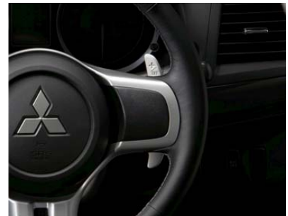
The TC-SST can be shifted manually with either the console mounted shifter or the magnesium steering wheel shifter paddles (below).
